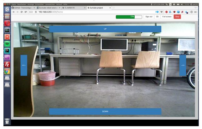
It is possible to check camera image, battery status and 3D computed pose. If you use PID controller (select on raspberry\_init.launch), you can also control robot using arrows on display.
